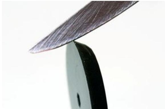
The coned side gives a slight waxy feeling. Cleaning and after-curing might solve this. For the initial process, this is not an important issue. I need to discover the safe limits for the exposuretime "Burn-in"-layers. The same object got printed over and over again while decreasing exposuretime. The minimum acceptable I can reach is a whopping 13.5 seconds. This low value is far from expected.
